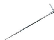
Earth contact test probe (80 cm)
